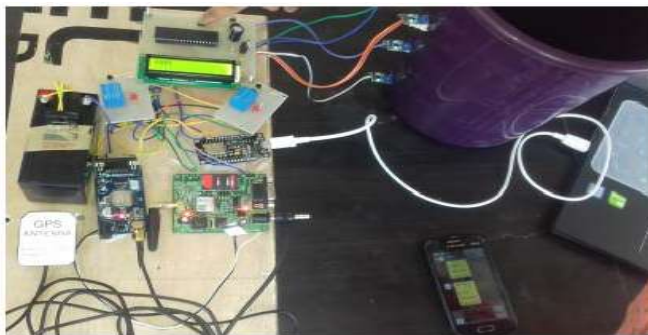
Fig. 4. Hardware setup with GPS and Wifi module
